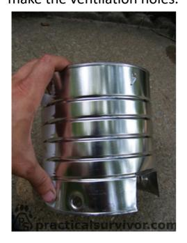
For this project we used a drill with a 1/2 inch drill bit to make the larger holes at the bottom of the can. If a drill is not available, the can needs to be supported by a piece of wood and a screwdriver or knife can be used to punch holes into the can.
