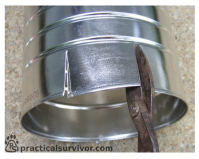
We then used the tin snips to cut a small door. This opening will be used to feed the fuel for the fire.
