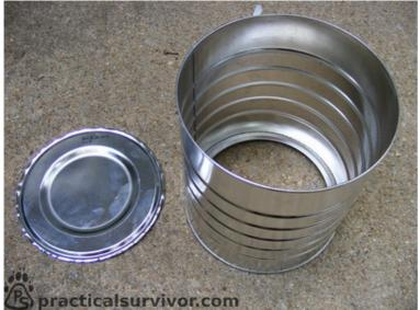
The top side of a coffee can is already opened. If the bottom is left on, we would not need the can opener for this project. Just make sure to drill extra holes in the bottom area of the can so the tinder gets proper ventilation.
