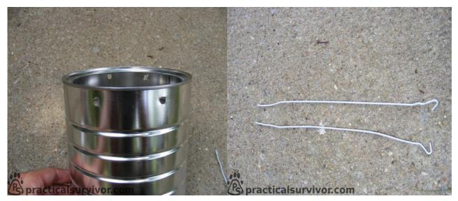
Four more holes need to be drilled along the top side. The holes will allow us to push the wire pieces we built using the coat hanger. Use wire cutters, a multi-tool, or just bend the hanger back and forth until it breaks.
